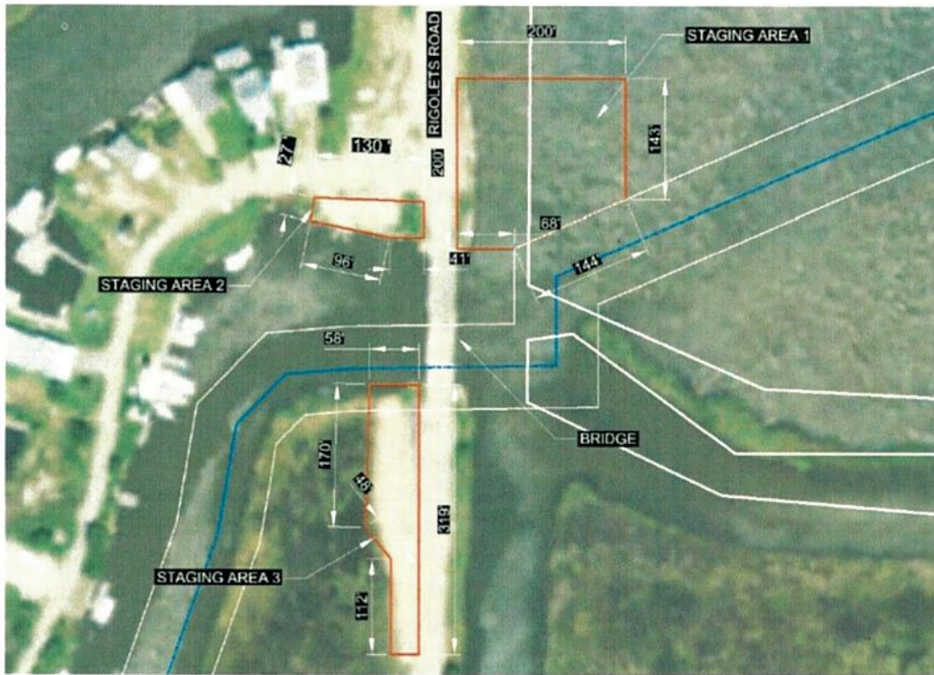
Figure 3: Staging Areas on Salt Bayou Road and Rigoletts/Highway 433 Additional Access Corridor (Southeast Corner of the Refuge) - For access into the marsh creation area.
